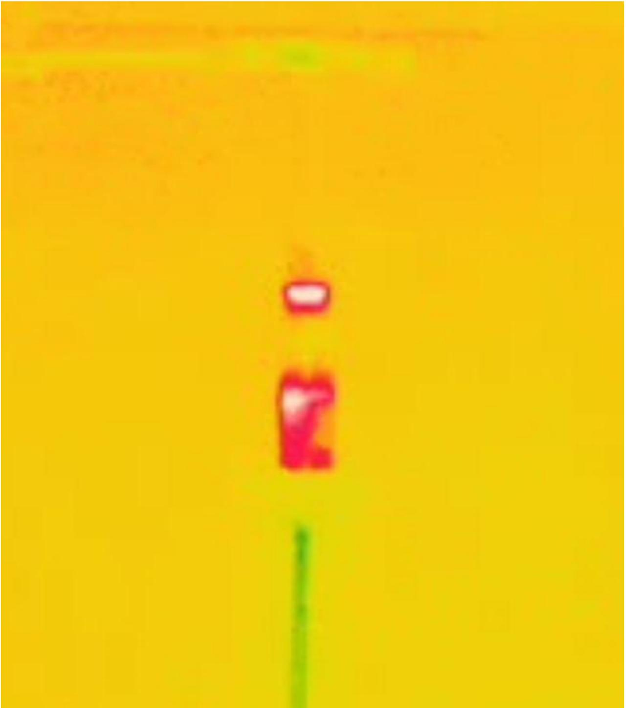
*Figure 5.8: IR image of an open vial containing ammonium hydroxide using the rainbow color palette. The ammonia vapors are harder to see with the rainbow or any of the other available color palettes.*
