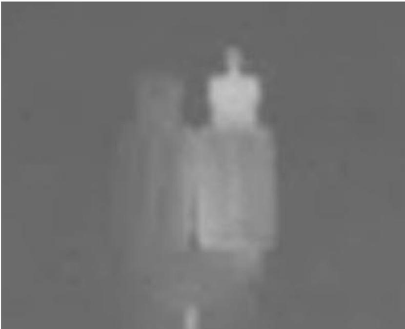
*Figure 5.37: An IR image of two 60 ml HDPE bottles, the one on the right containing 125 ppb TCE, and the one on the left containing air using the “white is hot” palette. The bottle containing TCE is lighter in color, while the background and the one containing air are darker in color.*
