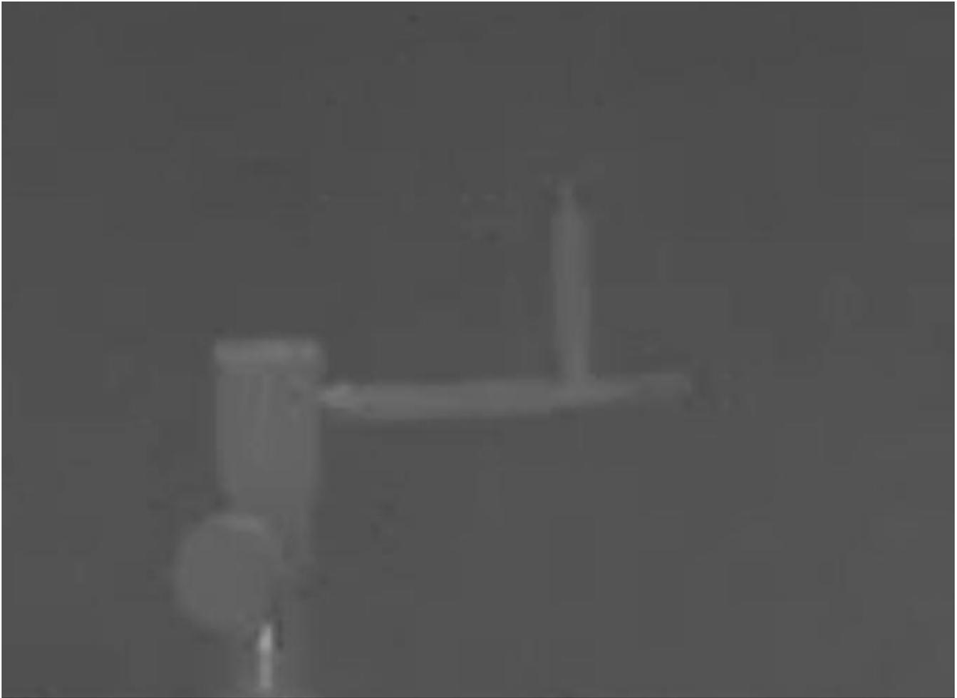
*Figure 5.11: IR image of the top of a TCE gas canister using the white is hot palette. TCE, if detected, would show up as a white cloud above the nozzle that is pointed upwards. A lack of a white cloud above the nozzle indicates the camera was not able to detect TCE.*
