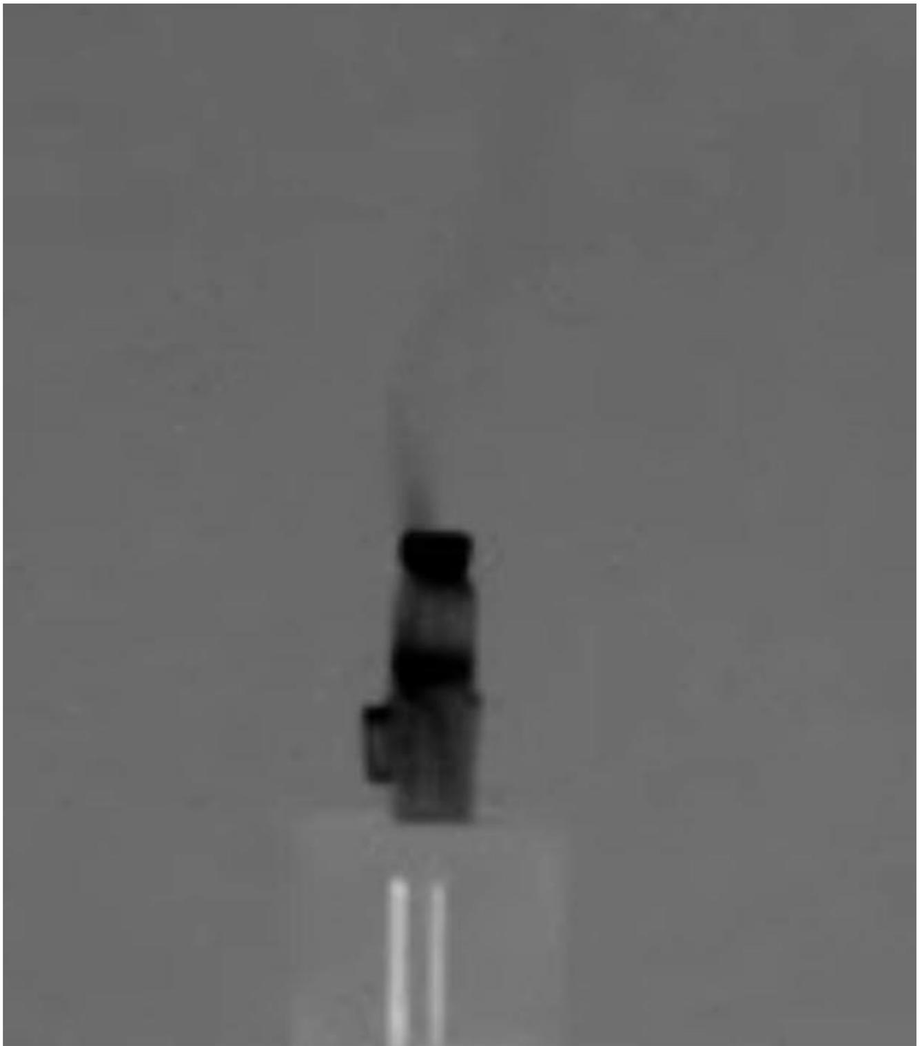
*Figure 5.6: IR image of an open vial containing ammonium hydroxide using the black is hot palette. A black plume is seen at the top of the vial as the liquid ammonium hydroxide vaporizes and is released into the air.*
