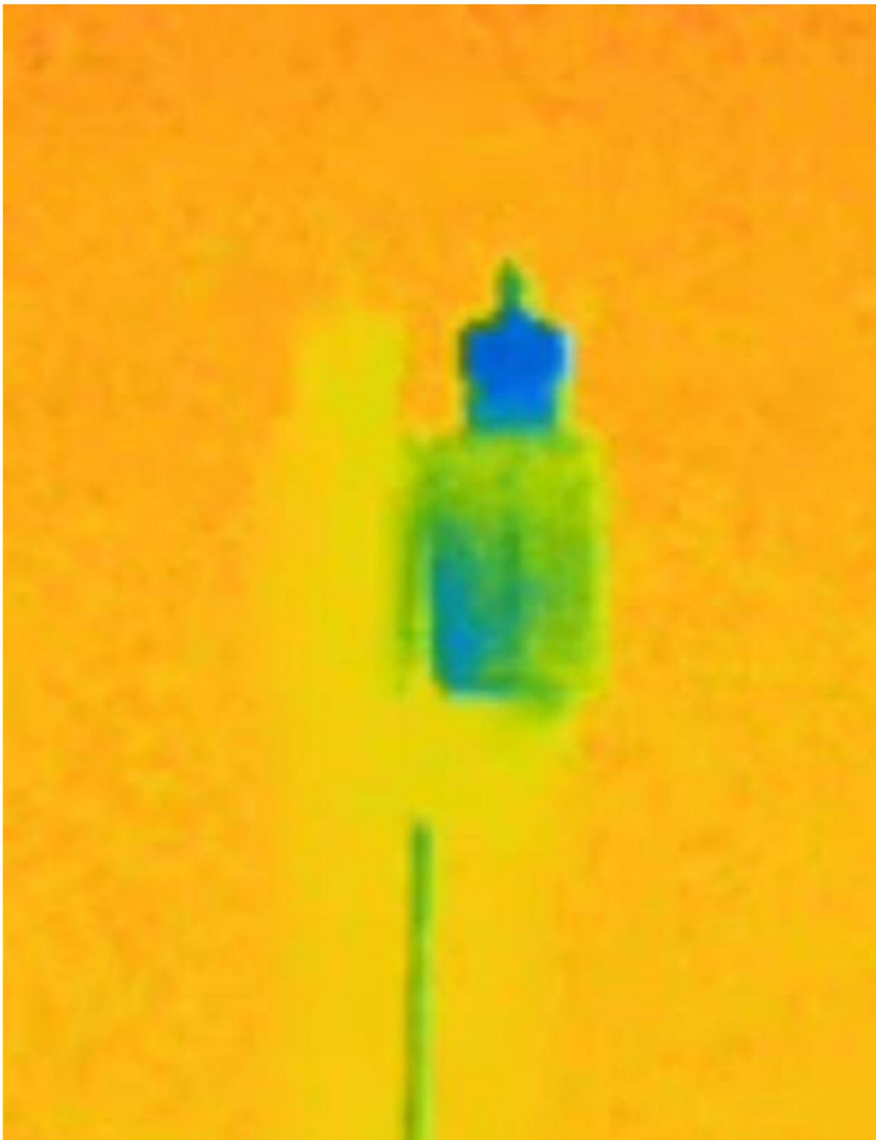
*Figure 5.35: An IR image of two 60 ml HDPE bottles, the one on the right containing 125 ppb TCE, and the one on the left containing air using the rainbow color palette. The bottle containing TCE is bluish green, while the one containing air is yellow.*
