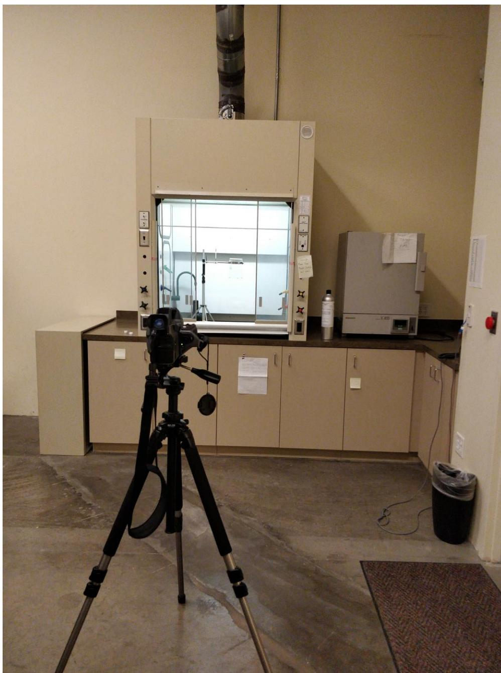
*Figure 3.3: Experiment set up at the EPA Region 6 Addison Facility. Gas canisters and vials containing chemicals such as ammonium hydroxide, dichloromethane, and hexanes were opened in the hood, and the camera was focused on the opening. The camera was placed exactly 8 feet from the hood.*
