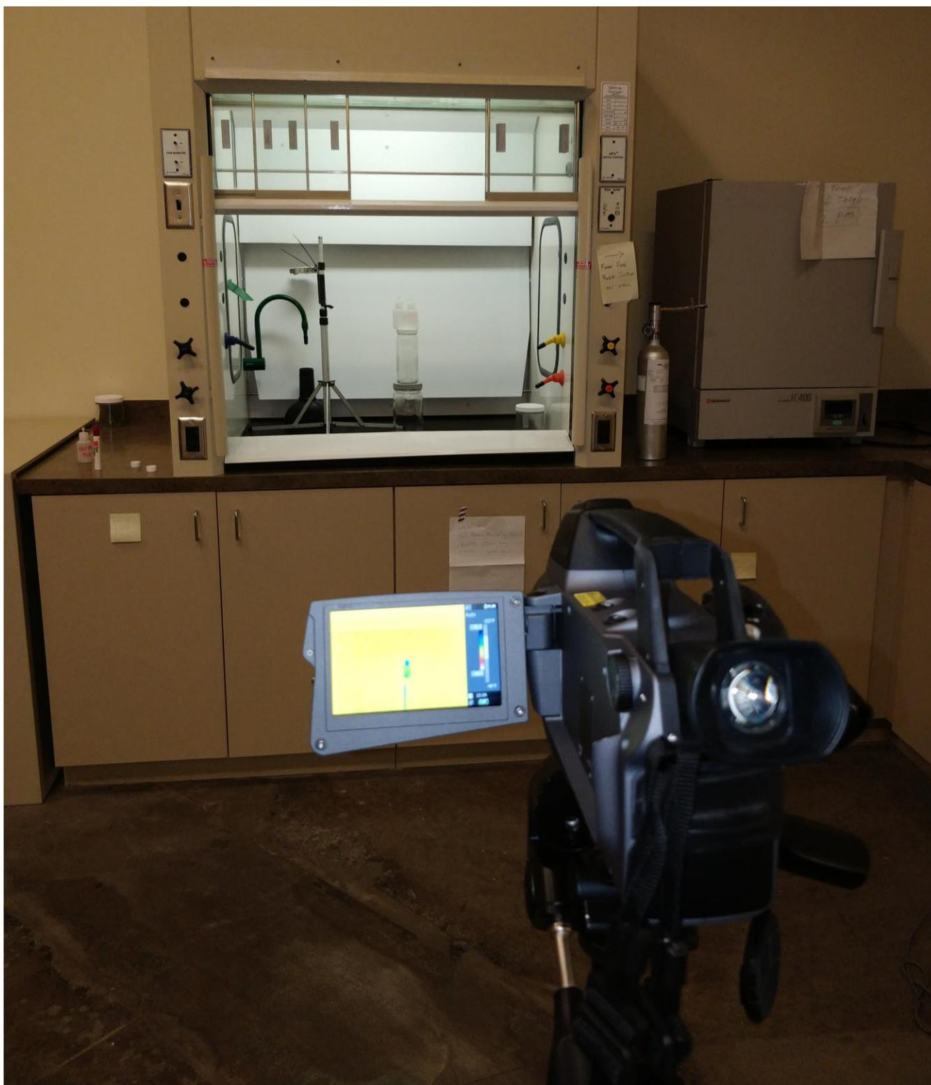
*Figure 5.38: A setup to detect TCE gas in a 60 ml HDPE bottle. Two bottles were placed side by side on top of two glass jars to keep the HDPE bottles in line with the camera lens. The bottle on the left contained air while the bottle on the right contained 125 ppb TCE. An IR image of the two bottles can be seen on the camera's LCD screen in the foreground.*
