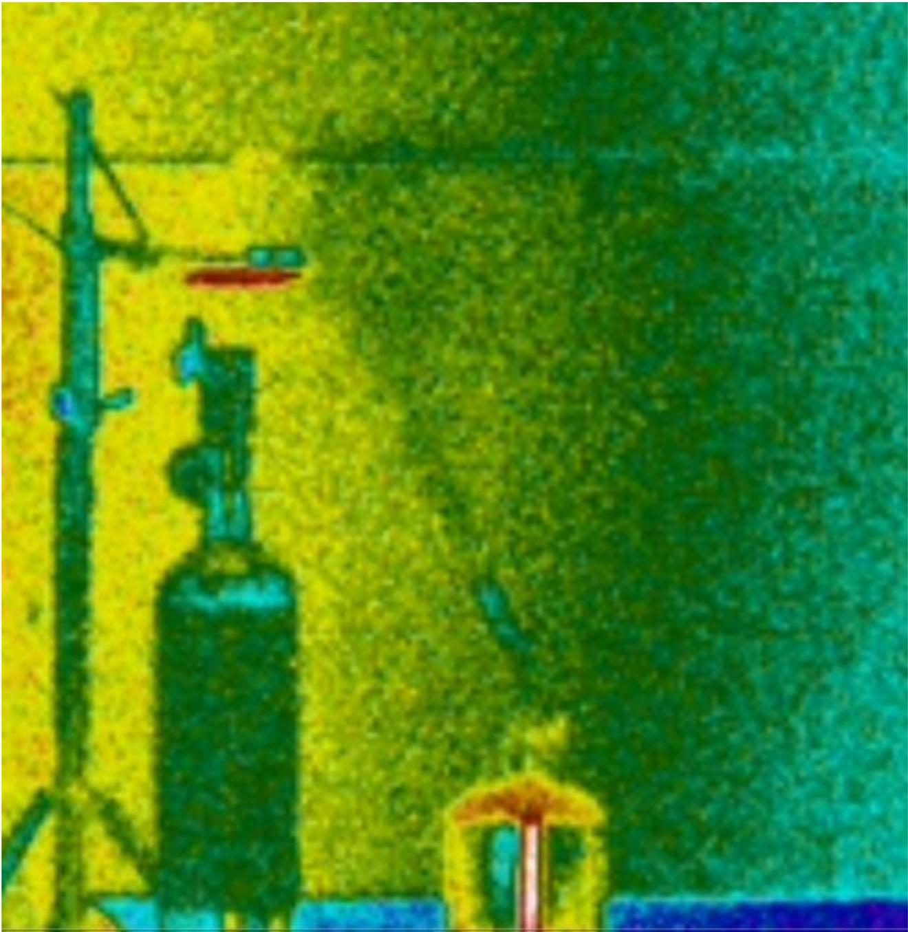
*Figure 5.5: IR image of an open propane tank using the rainbow color palette. The gas plume is seen as a black cloud against a yellow background.*
