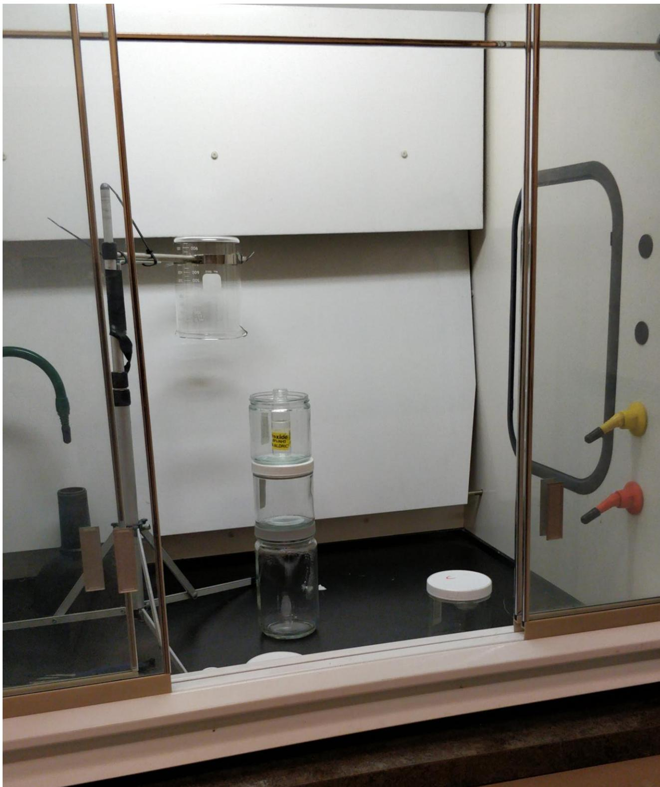
*Figure 5.27: An inverted beaker and other glass jars were tested to “capture” PCE or TCE gas. In the picture, an open bottle containing ammonium hydroxide that was placed inside one of the glass jars could not be “seen” by the FLIR GF-306 camera as the outside glass jar was made of borosilicate*
