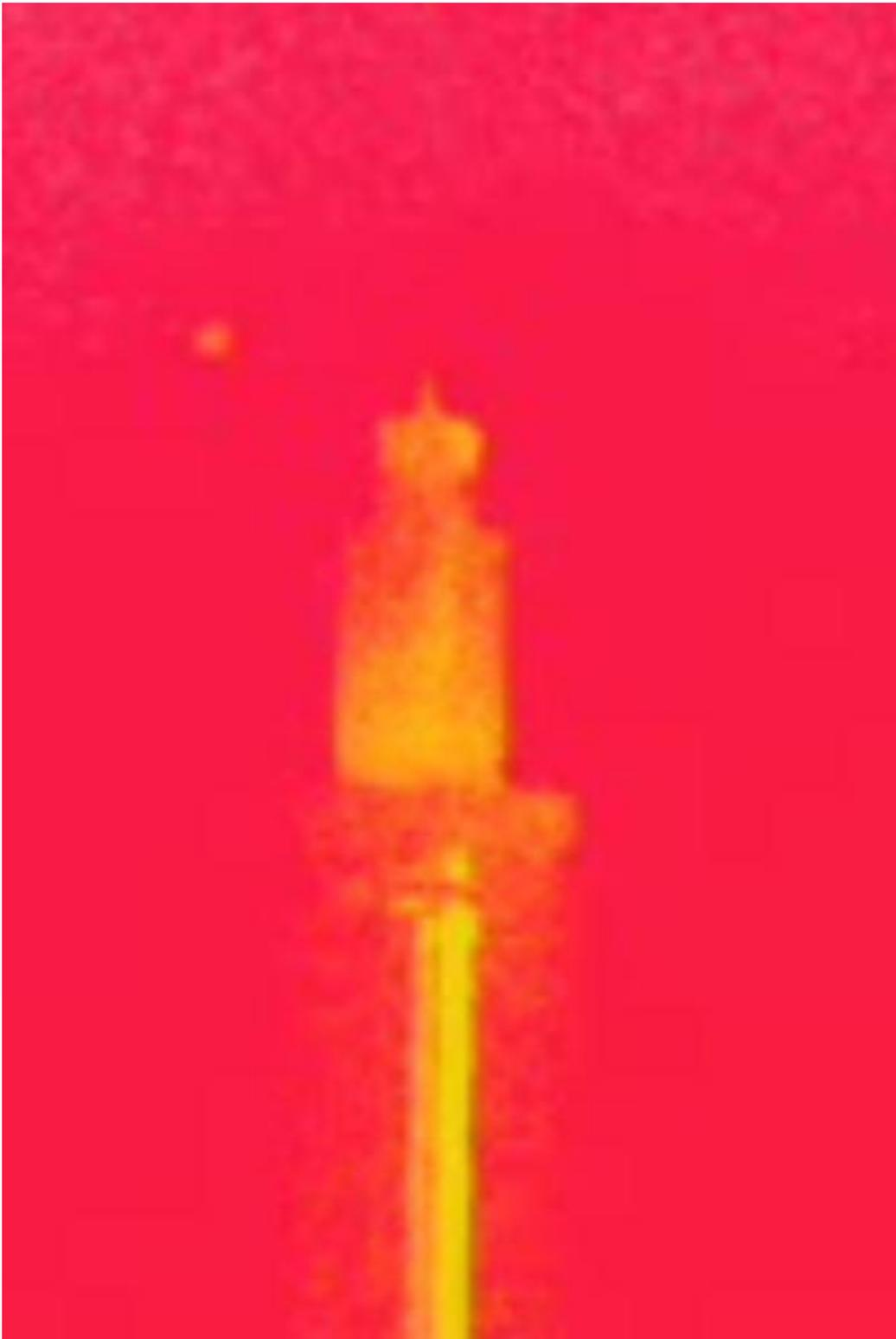
*Figure 5.31: An IR image of a 60 ml HDPE bottle containing a few drops of hexane using the rainbow color palette. The hexane and its vapor inside the HDPE bottle was not detected by the FLIR GF-306 camera.*
