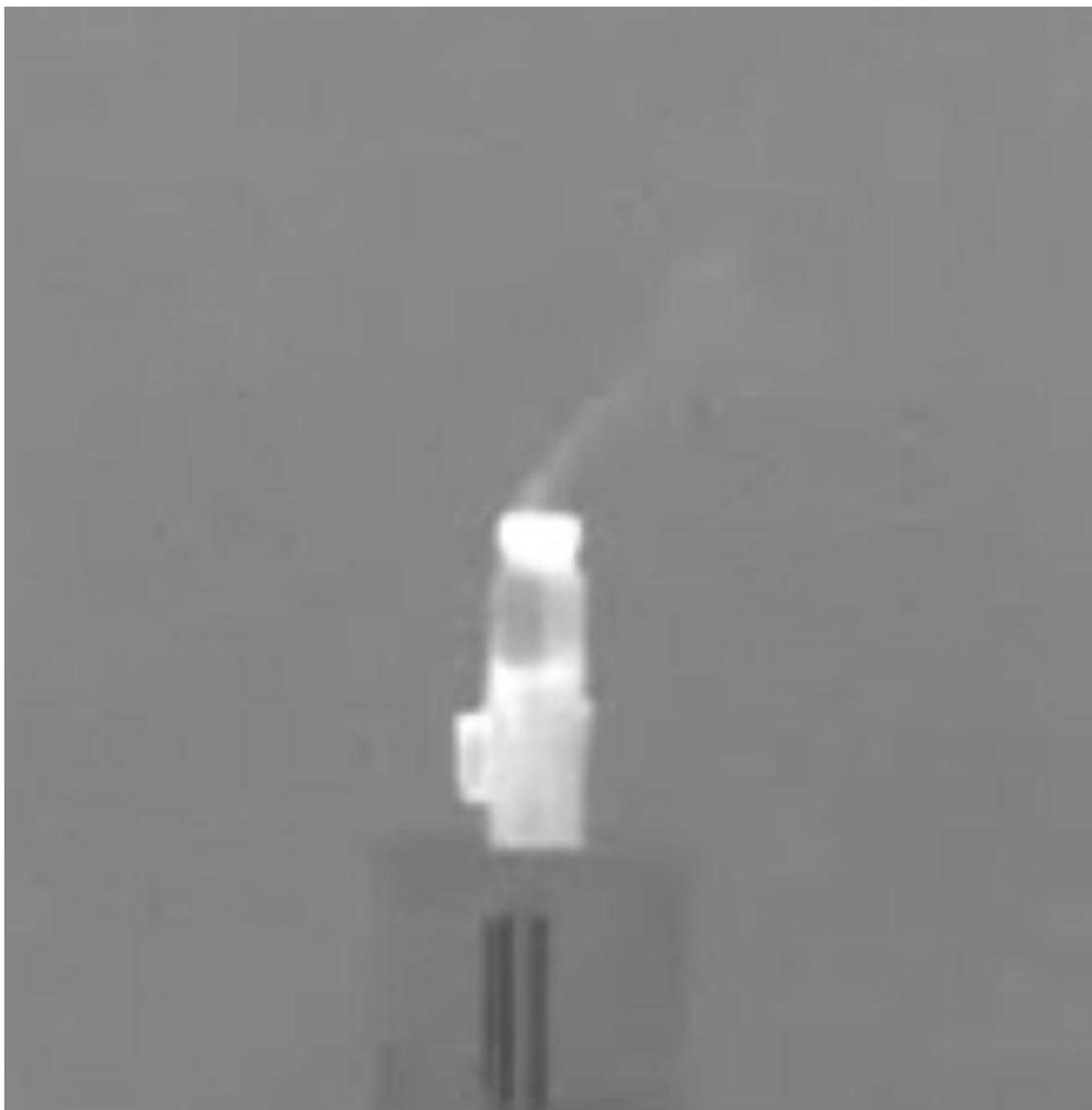
*Figure 5.7: IR image of an open vial containing ammonium hydroxide using the white is hot palette. A white plume is seen rising from the top of the vial.*
