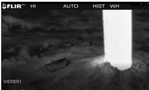
Vertical Wellhead Area Fugitive Emissions
