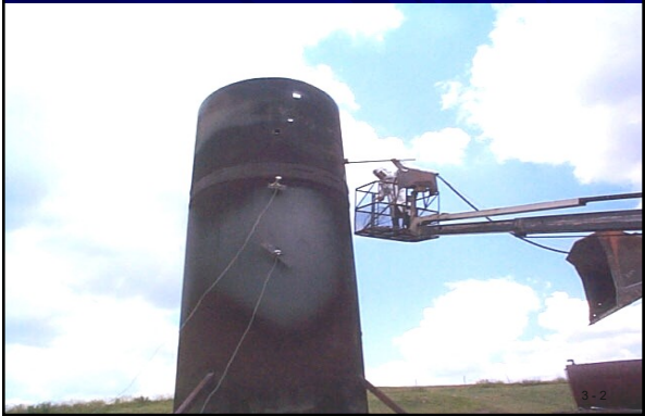
Sampling At a Landfill Enclosed Flare
