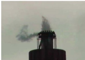
Poorly Operating Over Steam Flare - Low Combustion Efficiency
