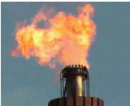
Well Operating Flare - High Combustion Efficiency
