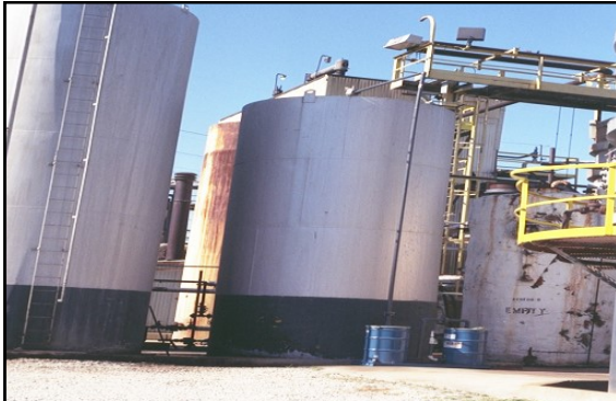
Non-Regenerative Carbon Adsorption Drums controlling mercaptan odors from re-refined crankcase oil product 4 - 109
