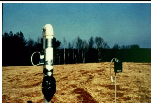
Encapsulated Vent Tube Sampling for PCBs Utilizing EPA Compendium Method TO-10A. (Note Portable Monitor to the Right of the Vent Tube for Ambient Monitoring of Emissions During Normal Vent Tube Emissions.) 10-60
