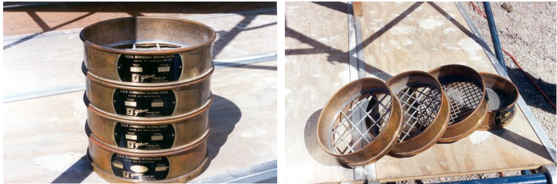
Figure 3-2. ASTM Sieves, Separated and Stacked for Shaking
