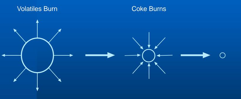
Coal Particle or Oil Droplet Evaporates Coke (Carbon)
