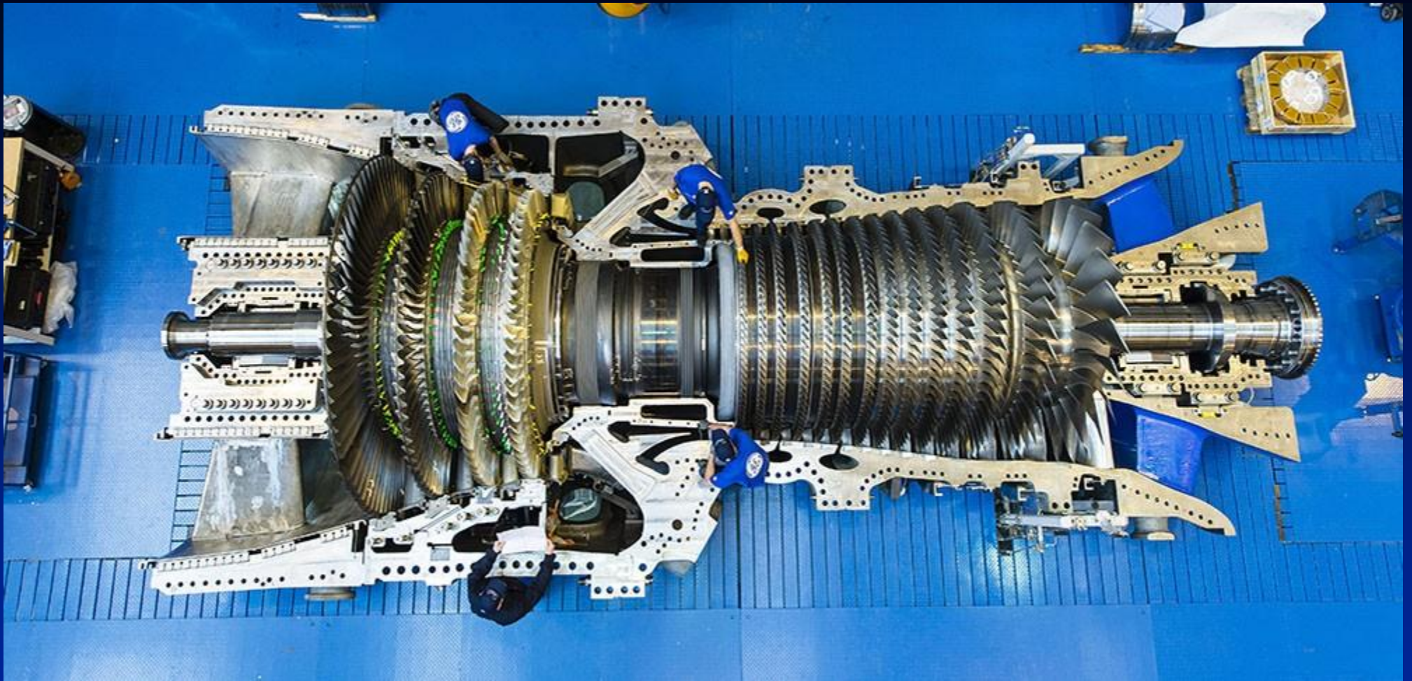
General Electric 9HA (397 MW – 532KHP)
