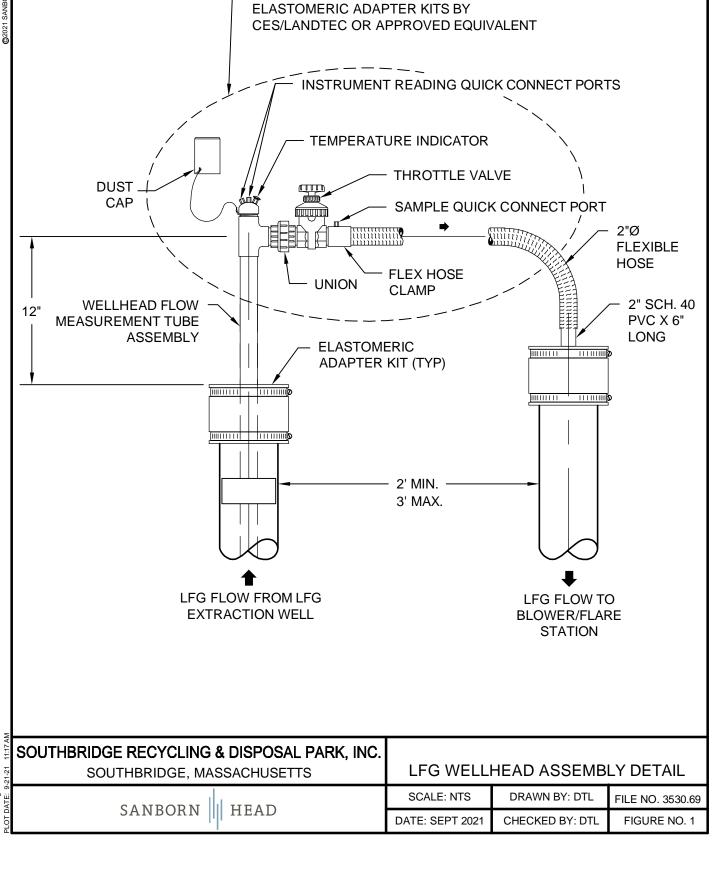
2" VERTICAL ACCU-FLO WELLHEAD WITH
