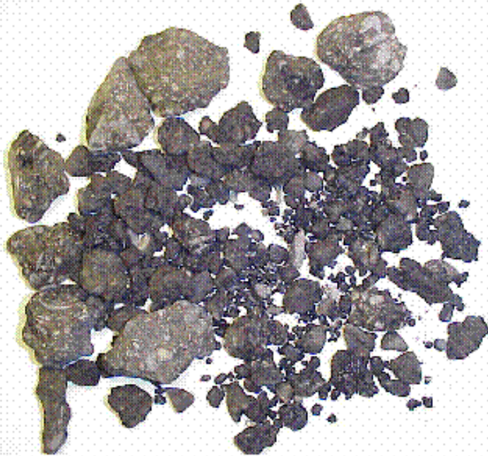
Figure 2.16: RAP in Aggregate-Sized Chunks
