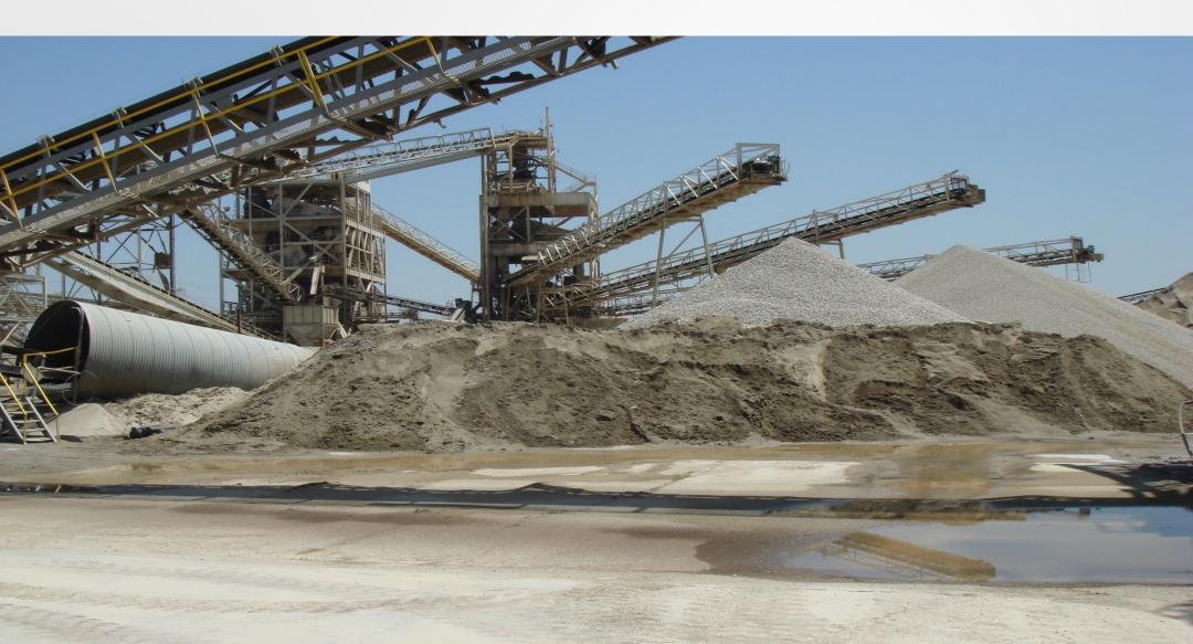
Concrete Batching: Aggregate Conveyors
